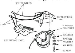
3.Install the receiving unit into hanger bracket.
